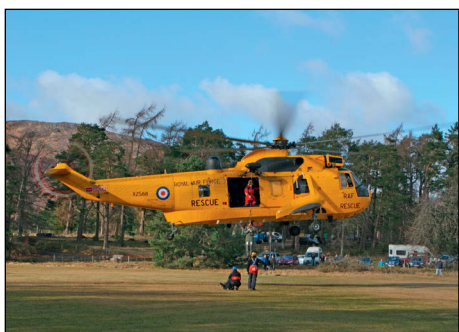
Figure 2.41 The upward force on the rotor is due to the force the rotor exerts on the air downward.
