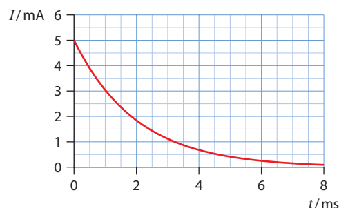
Figure 11.45 The variation of current with time for a discharging capacitor.
